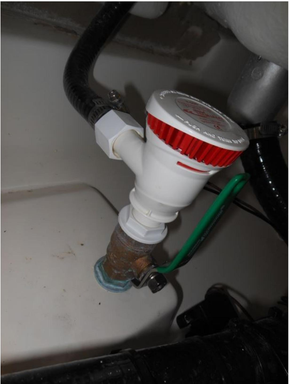
**Excessively leveraged raw water plumbing components are a damage control scenario waiting to happen.**
