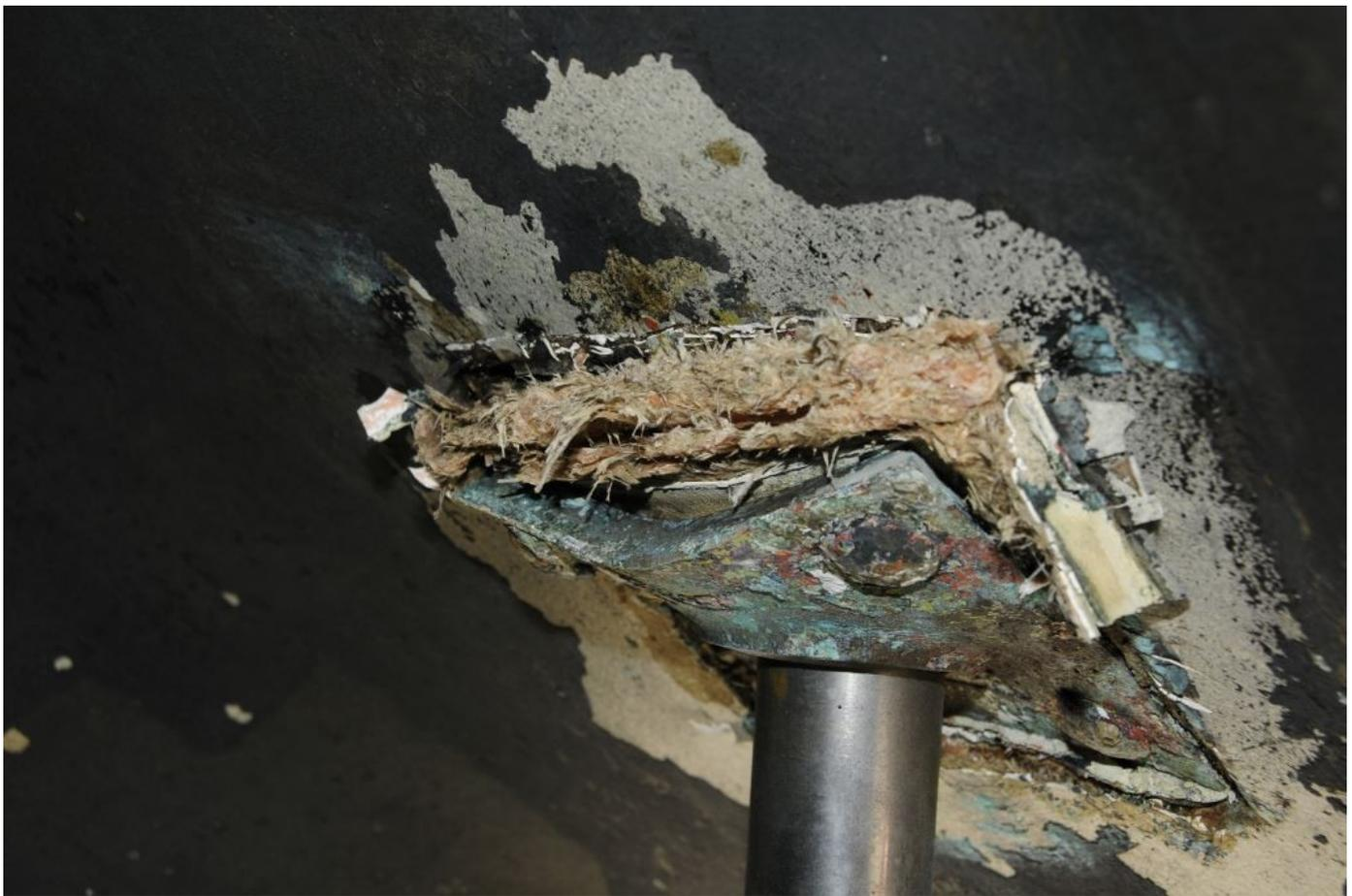
**Running gear components like struts, shaft logs and shafts are vulnerable to damage when running aground or striking submerged objects; which often leads to flooding.**
