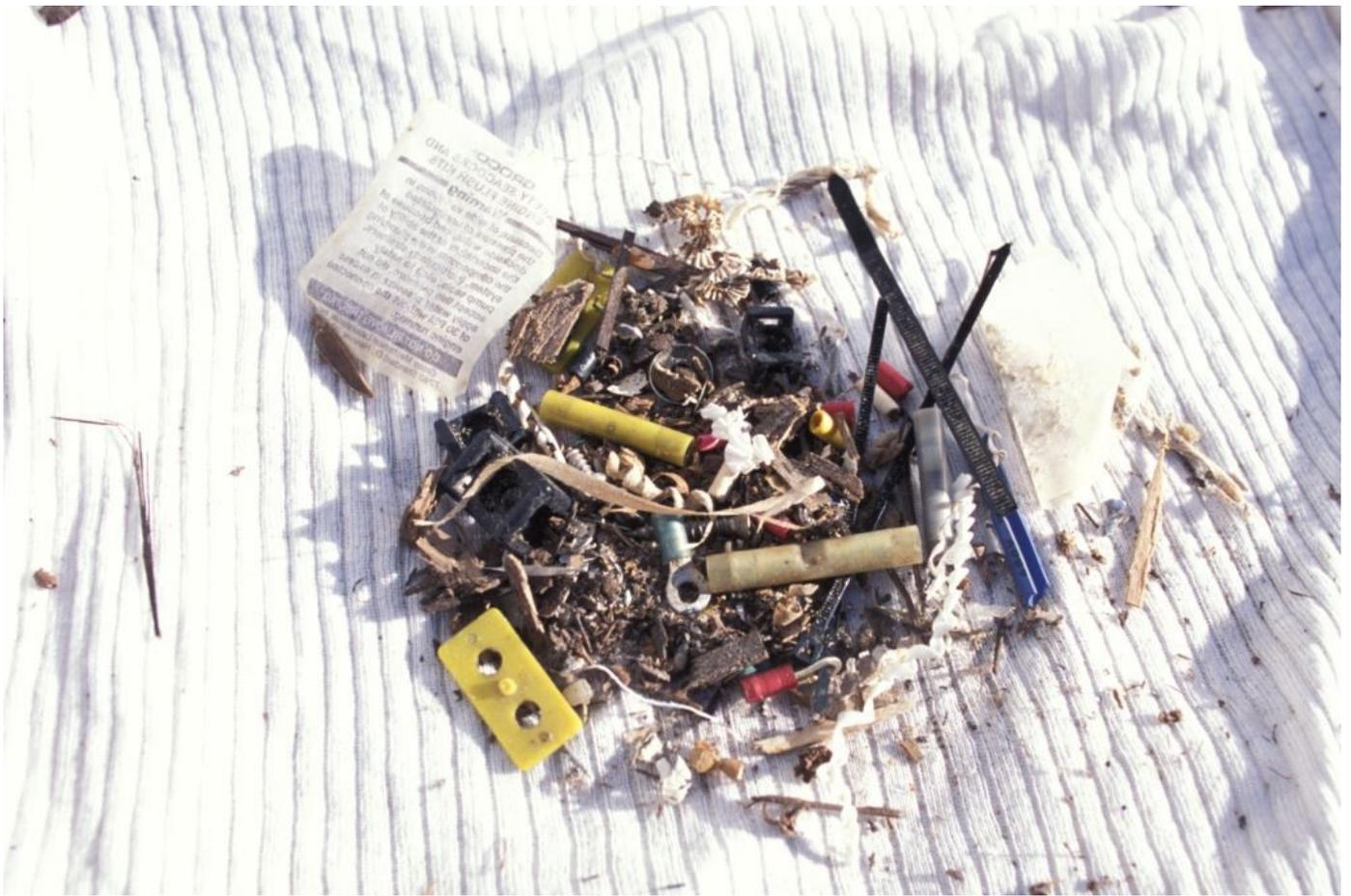
**When flooding occurs, trash and building debris are invariably washed into bilges, and bilge pumps. Keeping your bilges clean reduces the likelihood of clogged pump strainers.**
