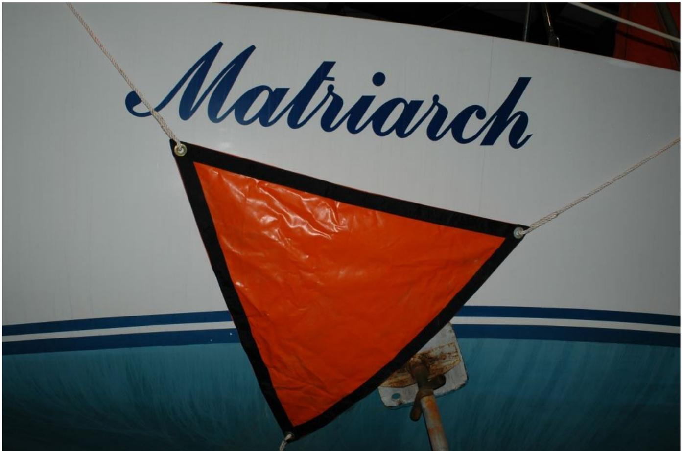
**Collision mats can prove useful in the event a damaged hull section cannot be accessed from the interior.**
