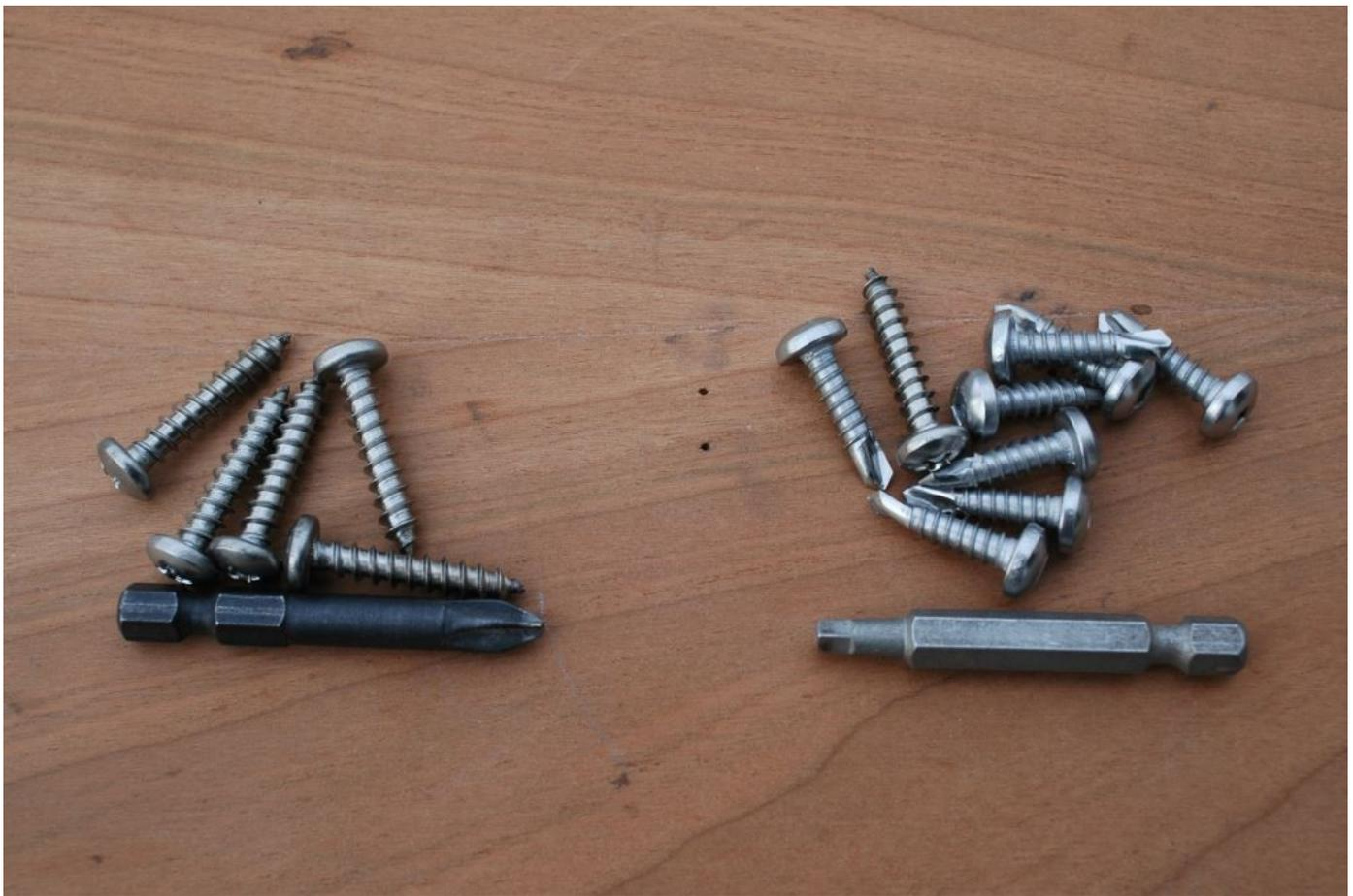
**Conventional Phillips head tapping screws, left, and cutting tip, square-drive screws, right, should be part of every damage control kit. Both must be stainless steel to ensure they don't rust while in storage.**
