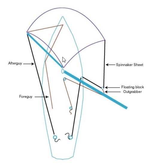
Outgrabber line leads from cabintop winch, forward to turning block at vang, aft along underside of boom, through turning block at mainsheet bails and dead ends at floating block. Floating snatch block pulls spinnaker sheet outboard to increase sheeting angle.
