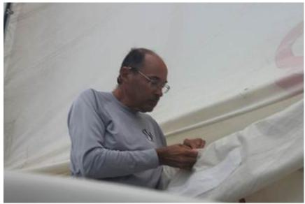
Sewing practice when the main split a seam a few days out of Kaneohe during the first long starboard tack. Needless to say my delivery sails are very old – over 30 years old - and need to be retired. We double reefed the main and sailed on. When we reached the light winds and flat seas of the high, we all took turns sewing the split seam – all 15 feet of triple stitched seam! Took us the better part of a day.
