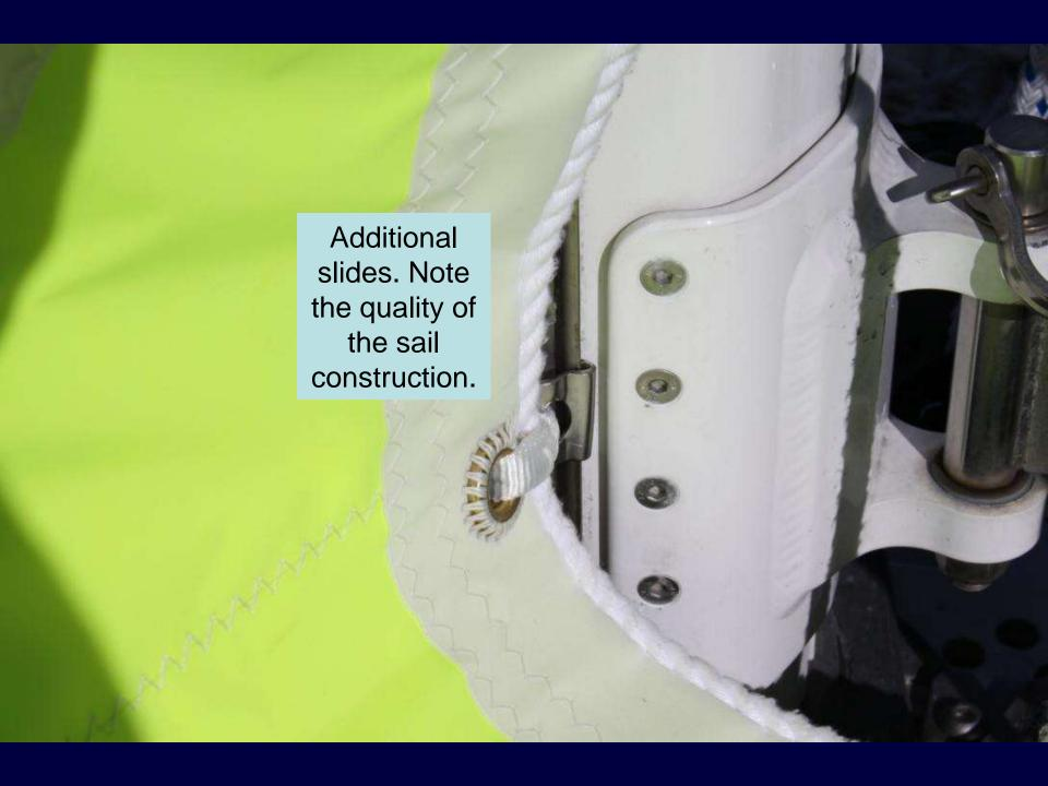
Storm trysail bent on and ready for hoisting.
